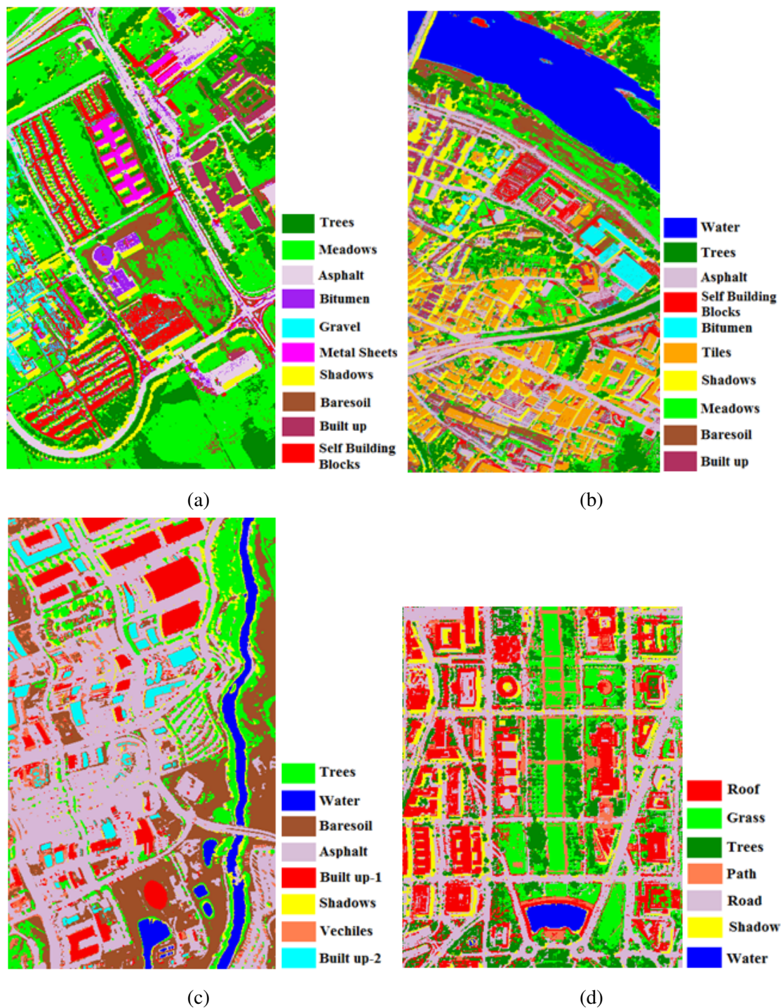
Figure 5.3: DCS-based classified images (best nontrainable combination function; the optimal dimension of the dimensionality reduction methods was estimated based on training samples classification): (a) ROSIS University, (b) ROSIS City of Pavia, (c) ProSpecTIR, and (d) HYDICE
