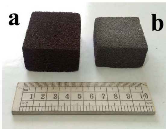
Fig 6.18 Photograph of (a) sucrose polymer-silicon powder composite foam and (b) SiC foam
