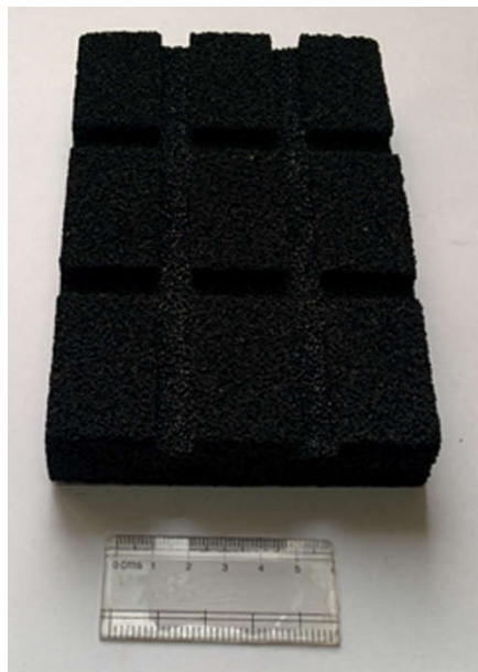
Fig 4.26 Photograph showing slots made by milling on rectangular carbon bonded alumina foam body in a conventional milling machine using a high speed steel tool
