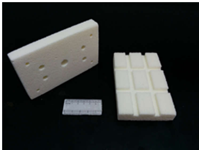
Fig 4.27 Photograph of alumina foam bodies prepared by carbon burnout and sintering of green machined carbon bonded alumina foam bodies. The slots are made by milling and holes are made by drilling.
