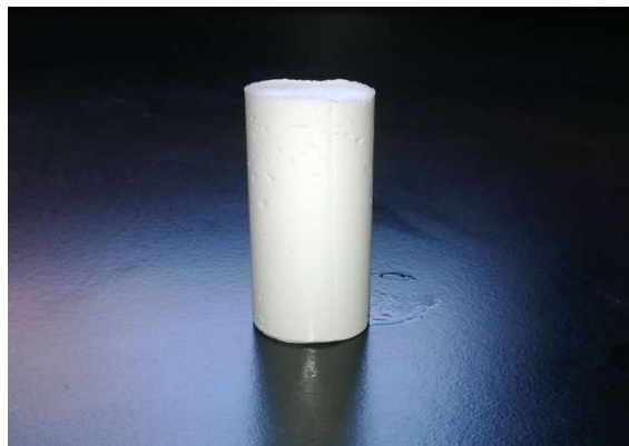
Fig 3.6 Photograph of a gelled emulsion body immediately after the mould removal
