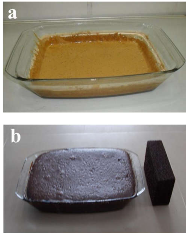
Fig 4.6 Photographs of (a) alumina powder dispersion in a 2.5 l glass tray and (b) the foam obtained by foaming at 150 °C.
