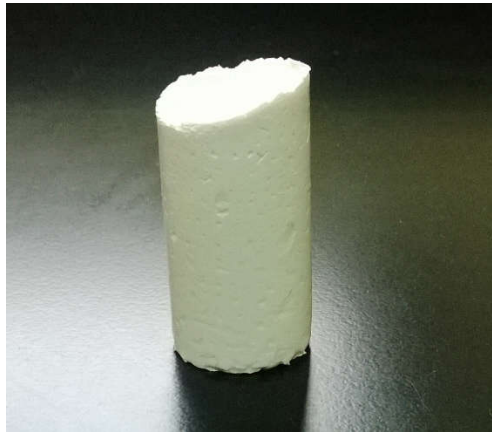
Fig 2.10 Photograph of a gelled emulsion body immediately after mould removal.
