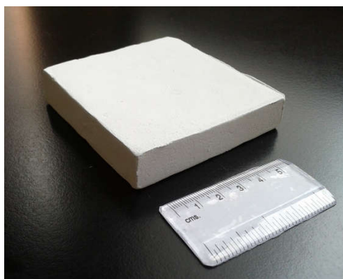
Fig 3.24 Photograph of a large sintered alumina foam body of 92.5 vol.% porosity.
