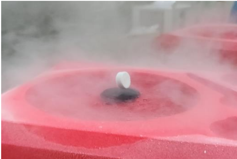
Figure: Quantum levitation with a superconductor cooled by liquid nitrogen at IIST, Physics Dept. The magnet is floating above YBCO, a high T_c Superconductor
