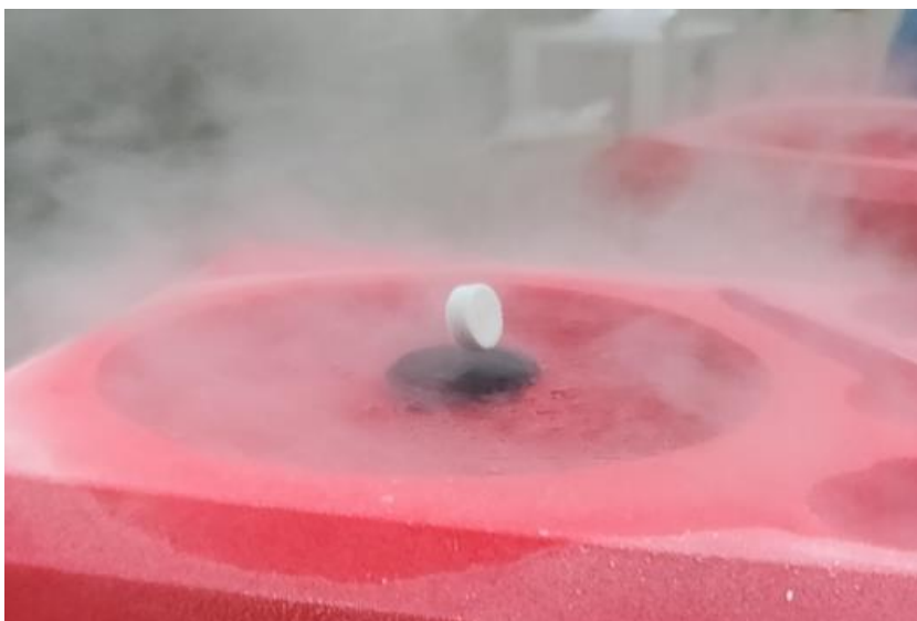
A magnet levitating above a superconductor cooled by liquid nitrogen at IIST, Physics Dept. A Nd magnet is floating above YBCO, a high T_c Superconductor
