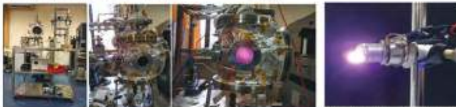
Design of Surface Discharge Sparkless Operates at 1 kV instead of 6 kV
