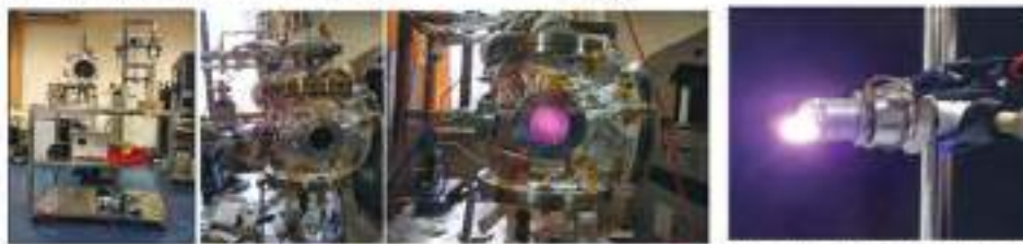
Design of Surface Discharge Sparkplugs Operates at 1 kV instead of 6 kV
