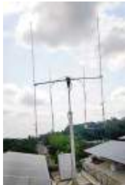
Standalone SDR-based VHF-UHF Ground Station Unit
