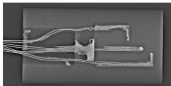
X-ray of instrumented specimen
