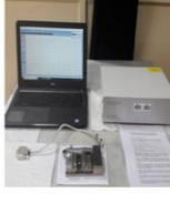
(b) Deben 2KN Micro Triaxial Tester.
