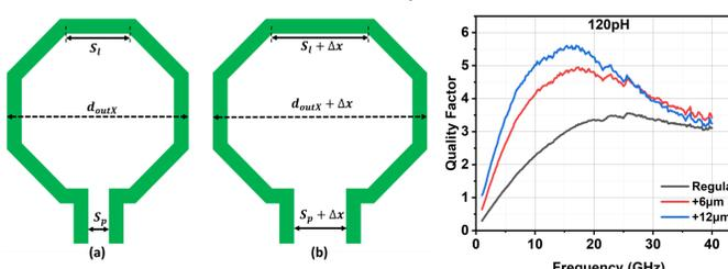
Fig.9 (a) Regular octagonal Inductor (b) Horizontal outer diameter expansion of the inductor
