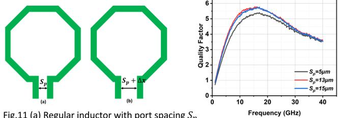
Fig.11 (a) Regular inductor with port spacing  $S_p$  (b) The inductor with increased port spacing  $S_p + \Delta x$
