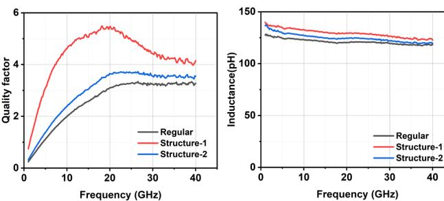
Fig.8. Plots of measured quality factor and inductance against frequency for the 120 pH regular inductor and the two inductors with n-well patterned structure-1 and structure-2.
