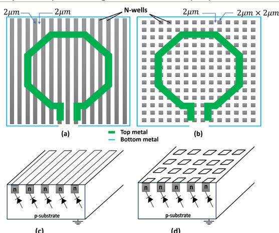
Fig. 5: Single turn octagonal spiral inductor with N-well patterned structures in the substrate. (a) Structure-1 with vertically oriented strips of n-well (b) Structure-2 with small islands of n-well (c) Cross-sectional view of structure-1 (d) Cross-sectional view of structure-2.
