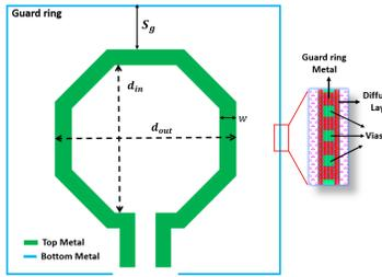
Fig.1. A typical octagonal single turn spiral inductor surrounded by guard ring.
