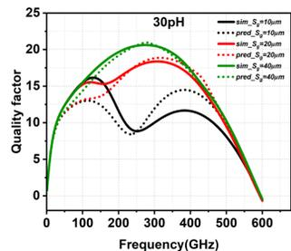
Fig.4. Plot of the simulated Q and predicted Q for 30pH inductor for various values of  $S_g$ .
