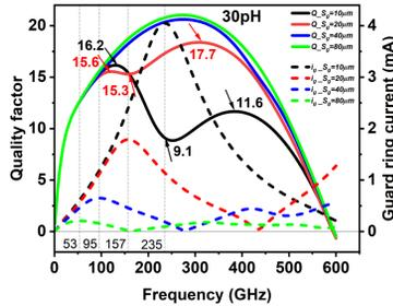
Fig.3. Plot of guard ring current and quality factor of the 30pH inductor with respect to frequency for various values of  $S_g$ .
