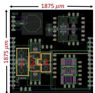
Fig. Micrograph of the chip, taped out in 65nm silicon CMOS.
