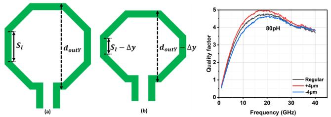
Fig.10 (a) Regular octagonal Inductor (b) Vertical outer diameter shrinking of the inductor
