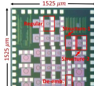
Fig.7. Micrograph of the chip, indicating and labelling the three test inductors referred, along with their de-embedding structure.
