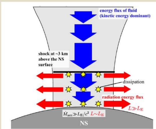
Fig 1: Schematic of supercritical accretion column (Kawashima et al 2016)
