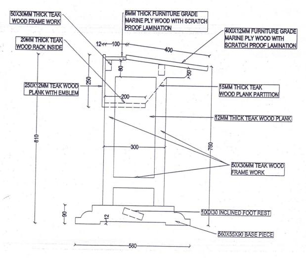
SECTIONAL ELEVATION (LENGTH 1.25H M.75H)
